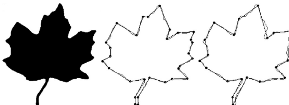
Fig 4. Masood's polygonal approximation for sample real shape
