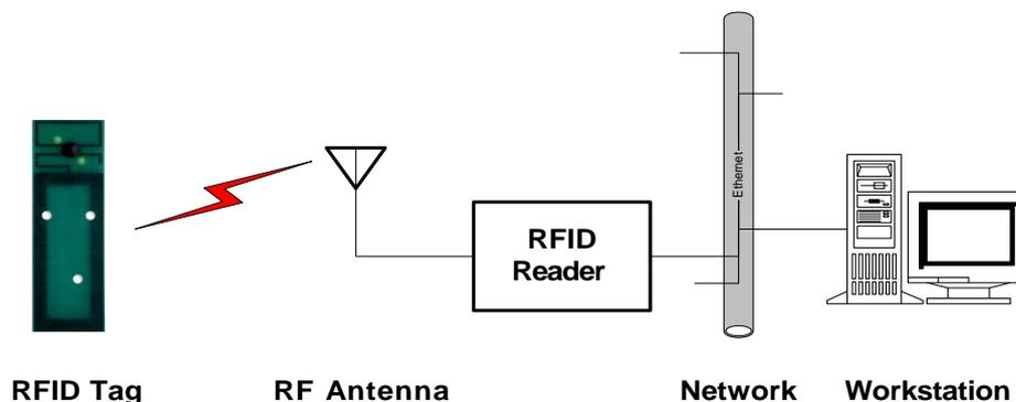
Figure 8: RFID system components
