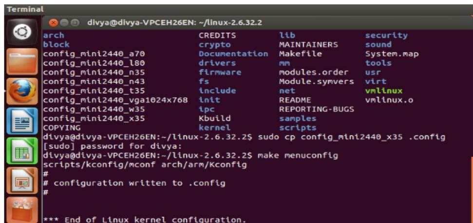
Figure 3: Configuring Linux kernel using make menuconfig
