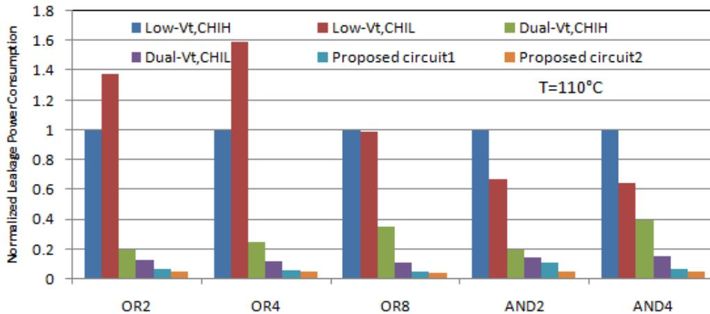
Figure 3.15 Comparison of the leakage power consumption of the proposed circuits and the existing techniques. The leakage power consumption is normalized to the leakage power of the standard low- $V_t$  technique with high inputs for each circuit.
