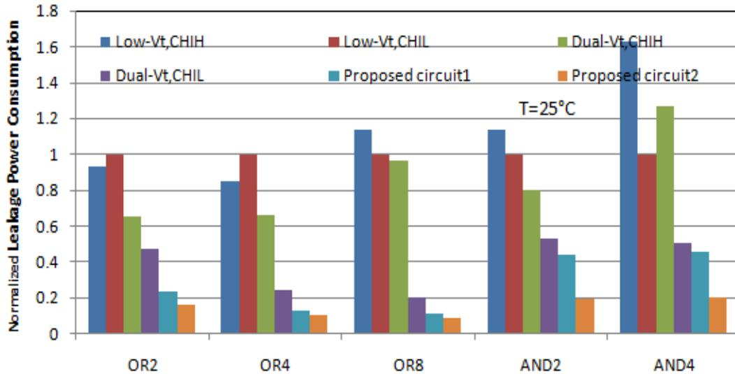
**Figure 3.14** Comparison of the leakage power consumption of the proposed circuits and the existing techniques at 25°C. The leakage power consumption is normalized to the leakage power of the standard low- $V_t$  technique with high inputs for each circuit.
