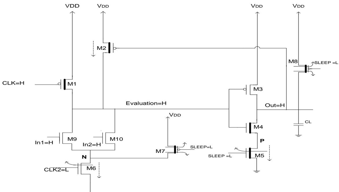
Figure 3 Variation of subthreshold and gate oxide leakage current conduction path in proposed circuit2.
