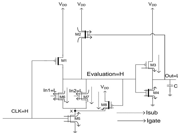
Figure. 2 Variation of subthreshold and gate oxide leakage current conduction path in proposed circuit1.
