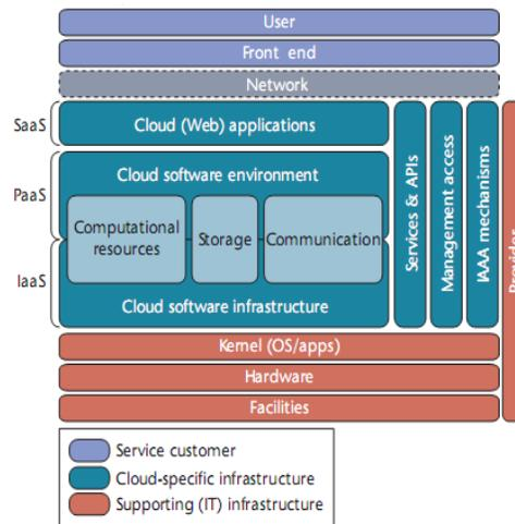
Fig. 4 Cloud Computing Architecture
