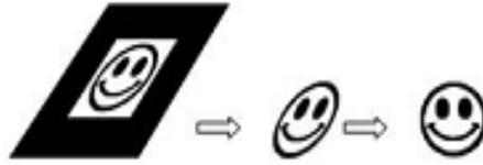
Fig 4: Procedure of unwrapping marker image to find ID
