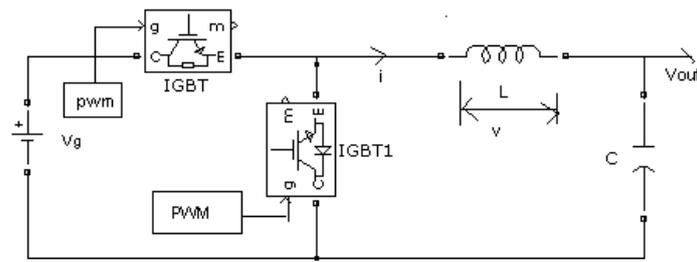
Fig. 1: Basic Synchronous buck converter
