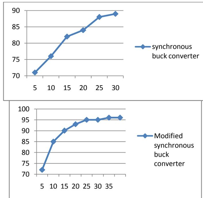
Fig. 8: Comparison of efficiency (Sync Buck Vs ZVT Sync Buck)
