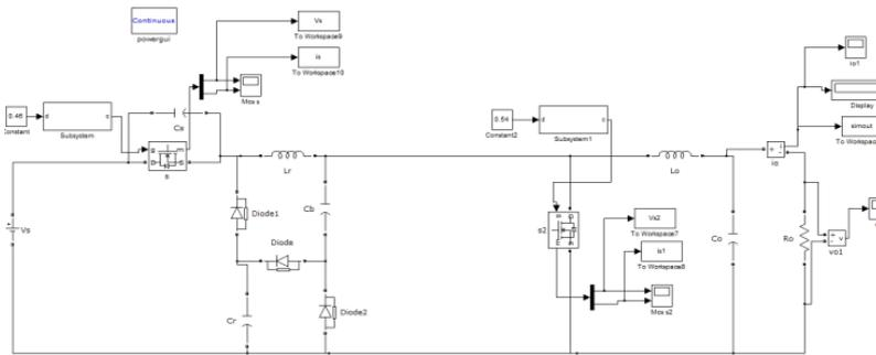
Fig. 5: Soft switching converter with Passive component
