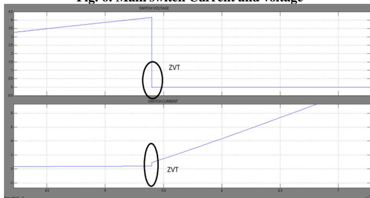
Fig. 7: Synchronous switch current and voltage
