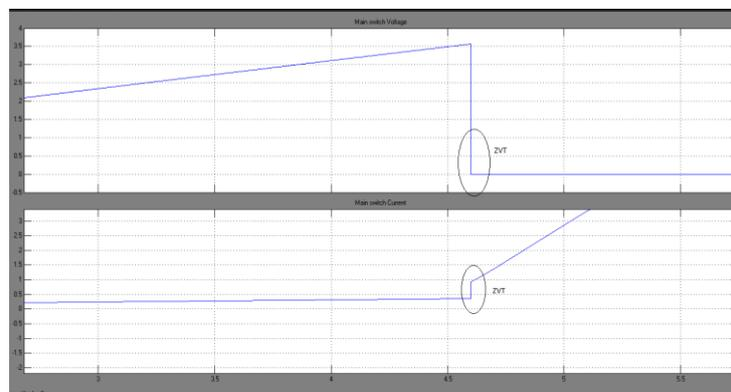
Fig. 6: Main switch Current and voltage
