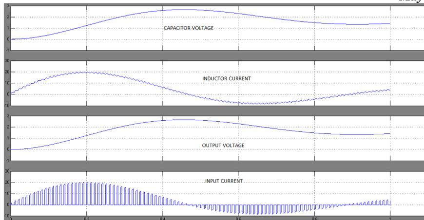
Fig. 3: simulated output of Synchronous Buck Converter
