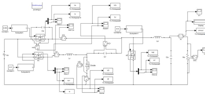
Fig. 4: Soft switching converter with Active component
