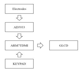
Once calibrated, the magnitude of the impedance and relative phase of the impedance at each frequency point along the sweep can be easily calculated. Using the real and imaginary register contents, this calculation is done off chip, which is read from the serial I2C interface. Also a 4x4 Keypad, 128x64 Graphical LCD are used for user access, REDDOT Electrodes are used for better measurement.
