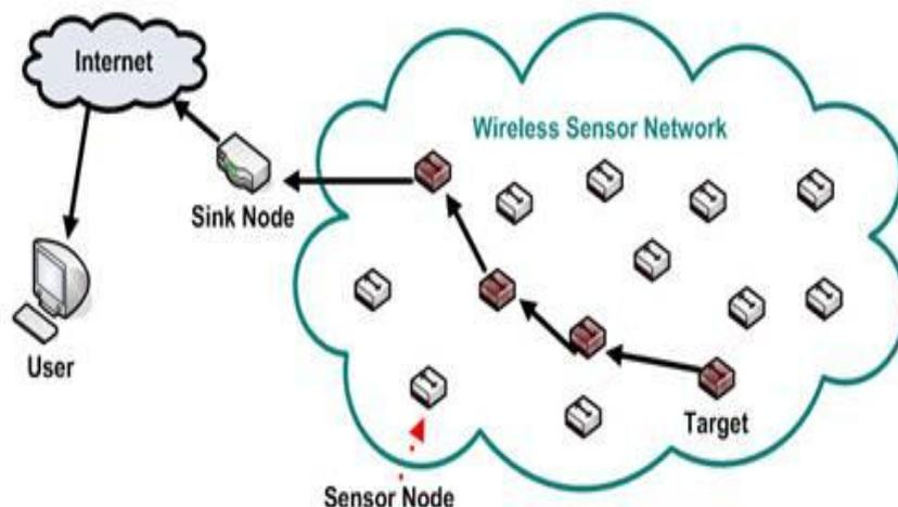
Fig. 1 Architecture of Wireless Sensor Network
