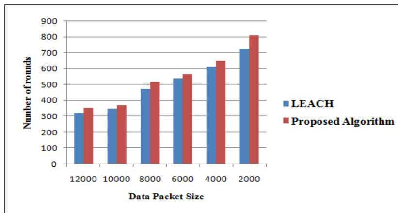
Fig. 6 Network lifetime with varying message size
