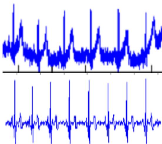
Figure2. Noisy (above) and noise free (below) ECG signal
