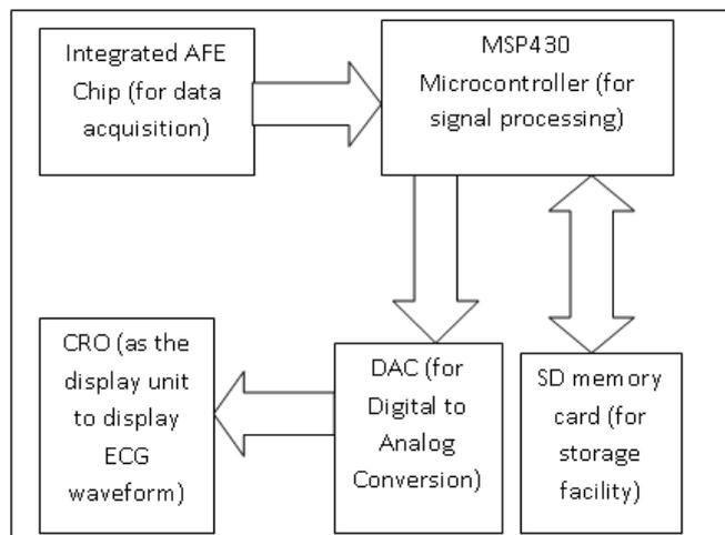
Figure3. Block Diagram of the ECG circuit
