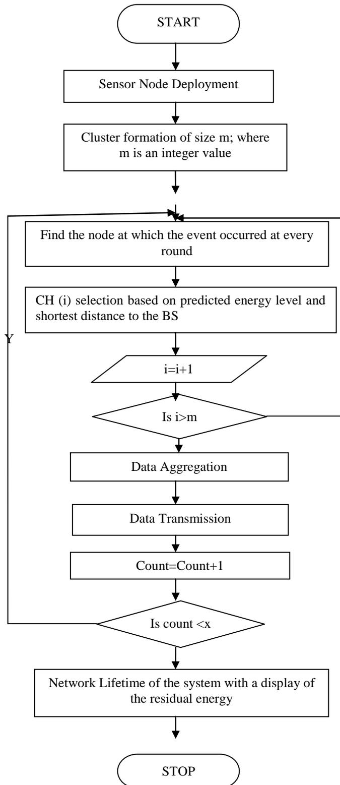
Fig 1. Flowchart of the proposed hierarchical routing technique.
