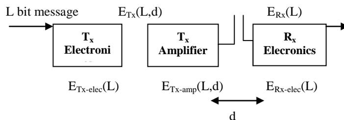
Fig1. Radio energy dissipation model
