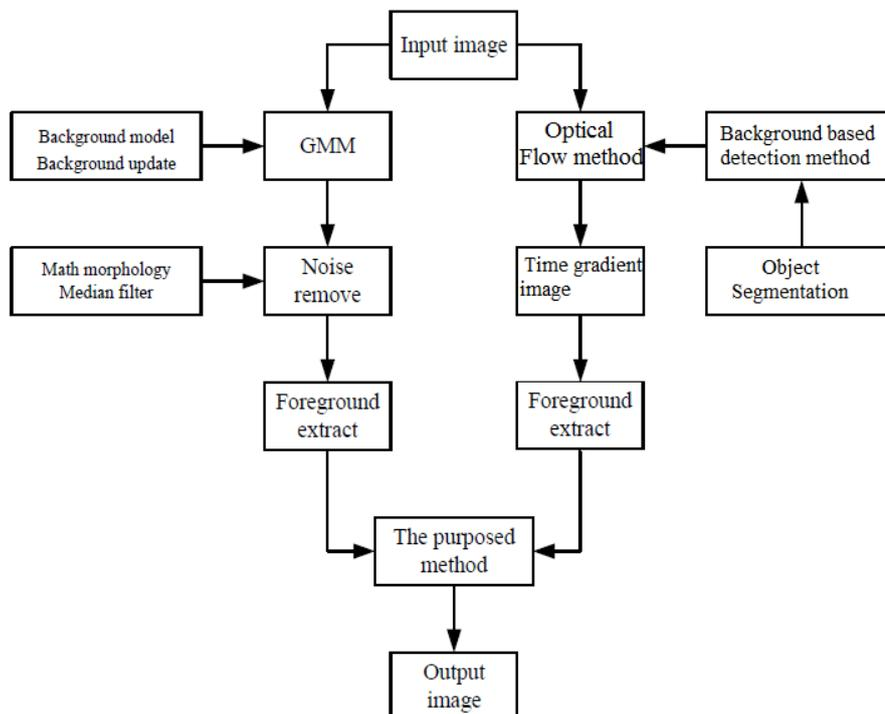
Fig. 1 Flow chart of the proposed object tracking
