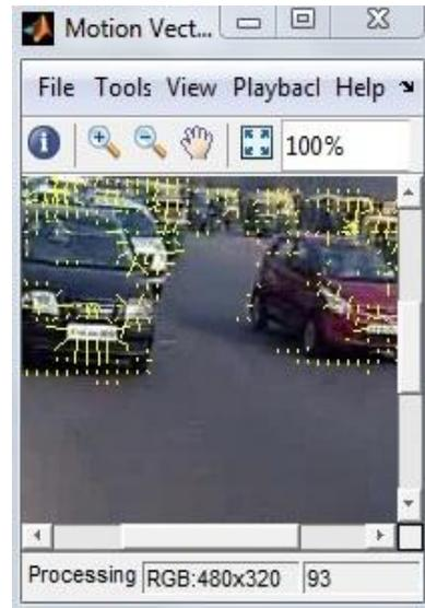
**Fig.3 Motion Vector (Using Optical Flow)**
