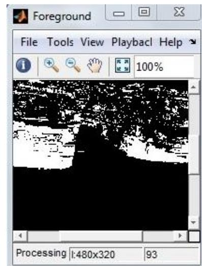
**Fig.5 Foreground Dtection (Using GMM)**
