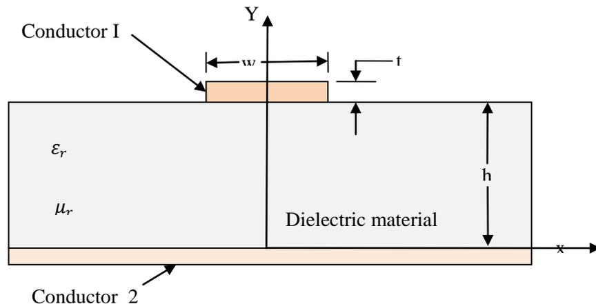
Fig. 2 Microstrip transmission line
