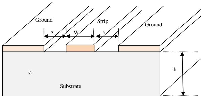
Fig. 3 coplanar waveguide of finite substrate.
