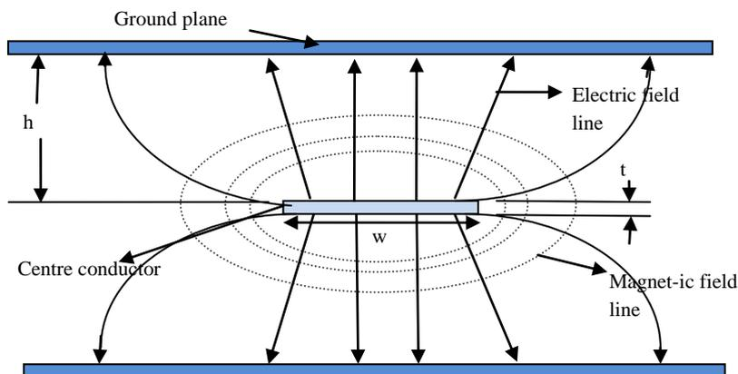
Fig. 1 Schematic diagram of stripline transmission line with field pattern.
