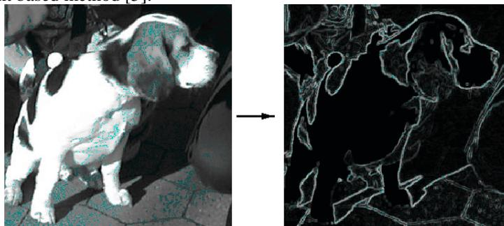
Fig 2. Edge based segmentation example [16]
