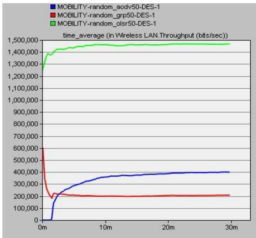
**Figure 2: Throughput comparison in routing protocols with random mobility with 50 nodes**
