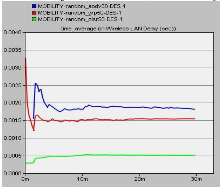
Figure 3: Delay comparison in routing protocols with random mobility with 50 nodes
