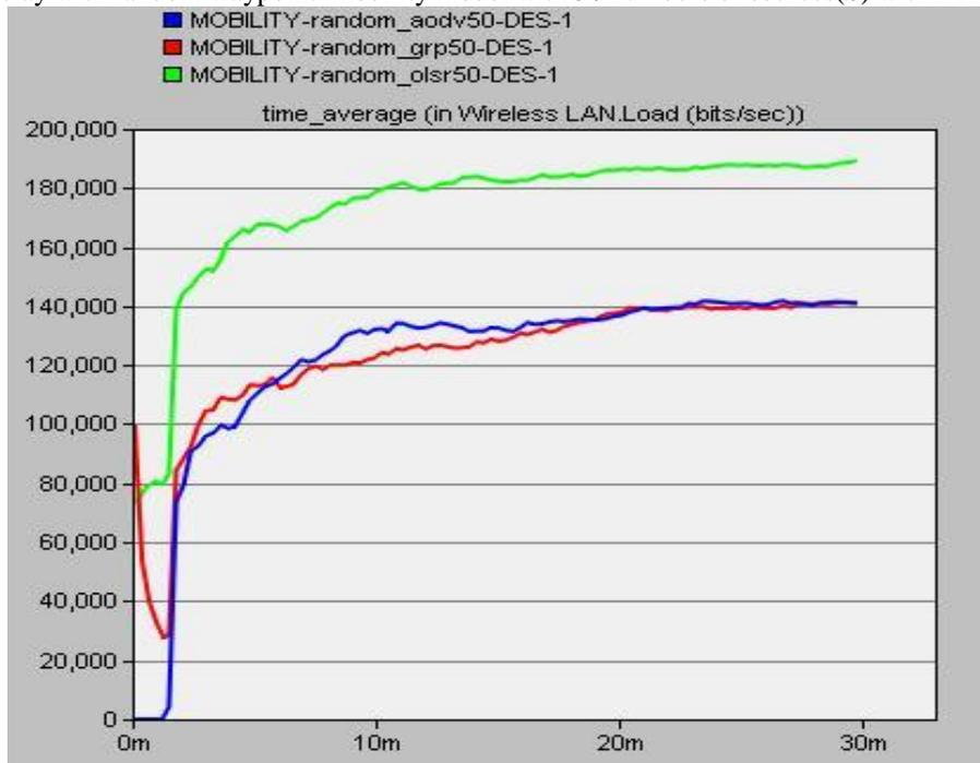
Figure 4: Network Load comparison in routing protocols with random mobility with 50 nodes
