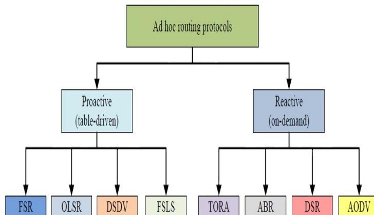
Figure 1: Classification of MANET Routing Protocols
