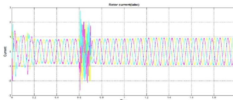
**Fig.6 (b) Rotor current during voltage sag (.6s to.7s)**
