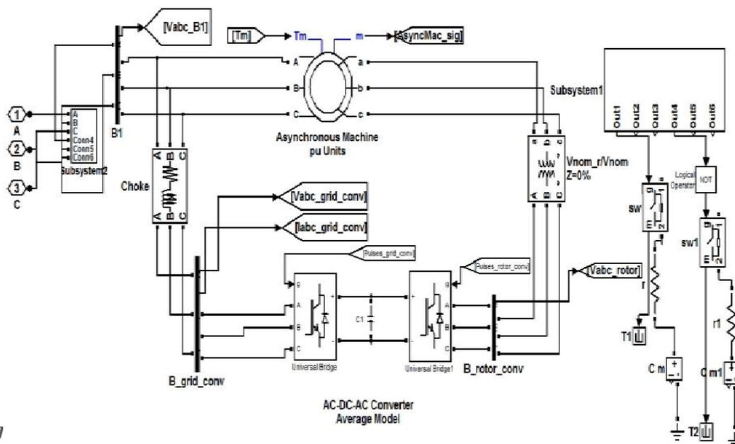
**Fig 4.Detailed simulink model of DFIG**
