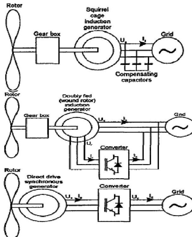
Fig2. Widely used contemporary wind turbine concepts
