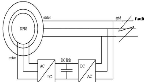
Fig 3 Block diagram of DFIG with fault at grid side
