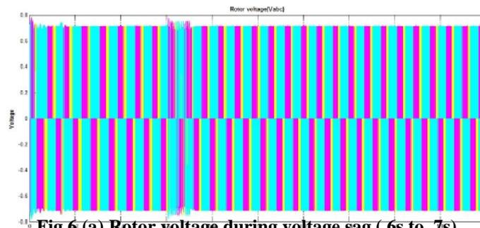
**Fig.6 (a) Rotor voltage during voltage sag (.6s to .7s)**
