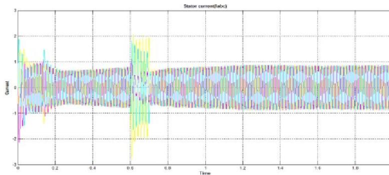
**Fig.5 (b) Stator current for dip .6s to .7s**
