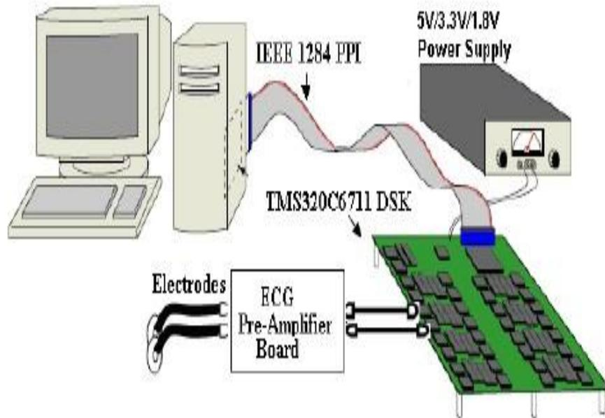
**Fig 2 DSP starter kit based ECG analysis setup**
