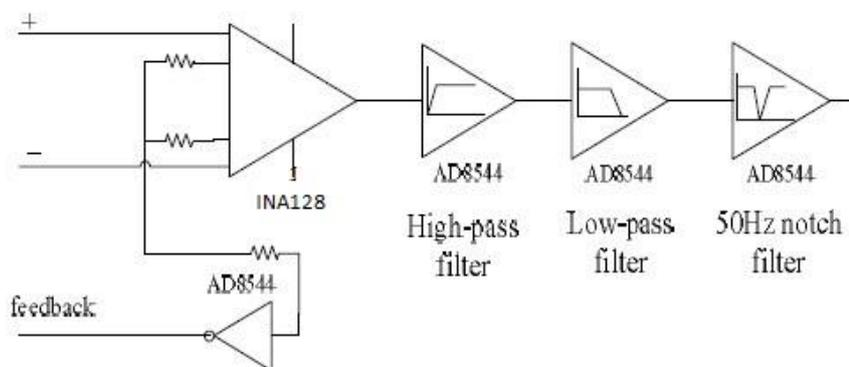
Fig 1 Analog front end unit (without ADC)
