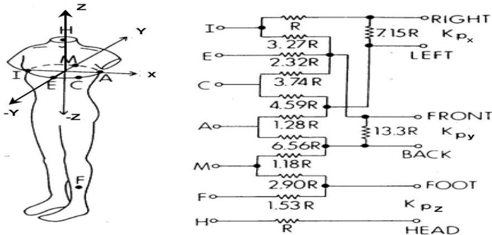
Fig 6 Frank electrode system to record the three-dimensional projection of the heart dipole
