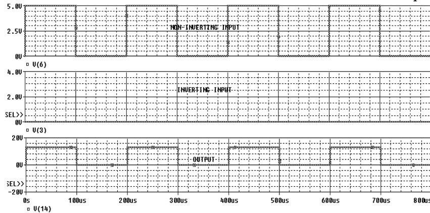
Figure 10: Simulation results of Non-Inverting Amplifier using CMOS
