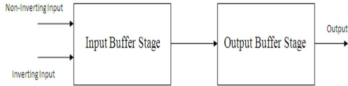
**Fig. 2: Block Diagram of CFOA using BJTs**
