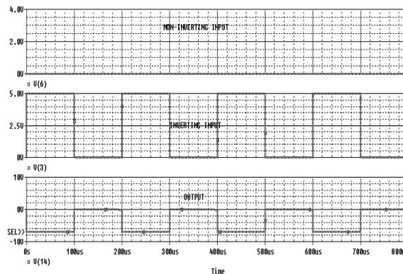
**Fig. 6: Simulation results of Inverting Amplifier using BJT**
