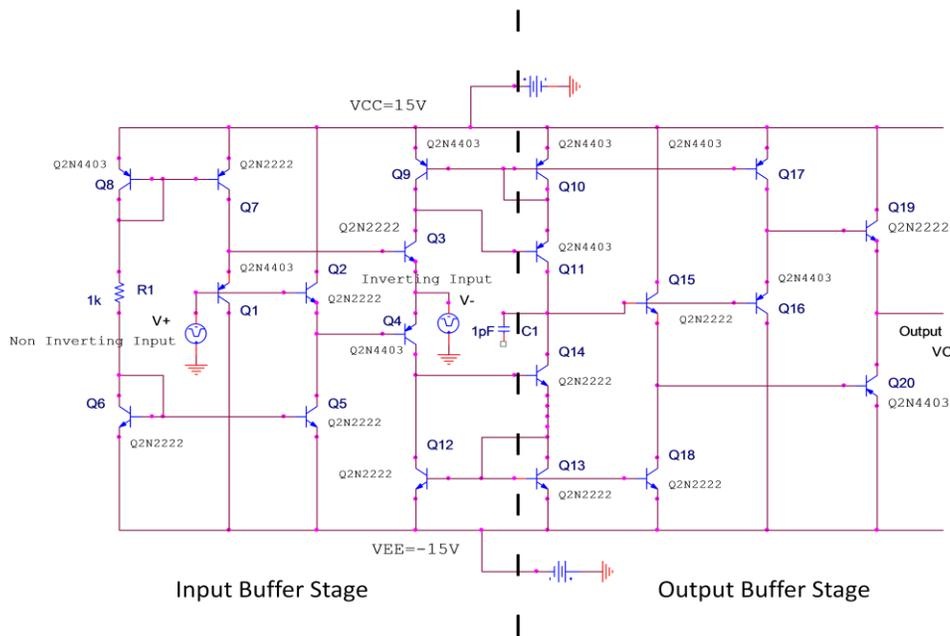
**Fig. 3: Operational Amplifier Using BJT**
