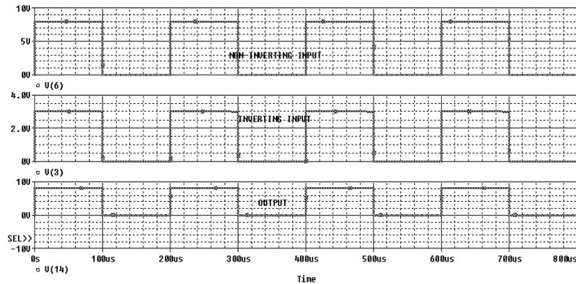
Figure 11: Simulation results of Differential Amplifier using CMOS
