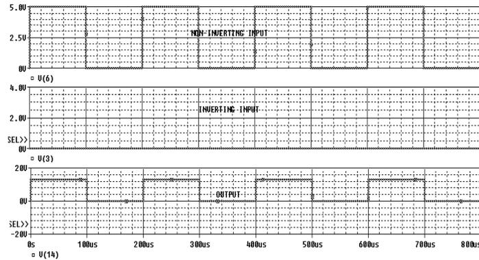
**Fig. 7: Simulation results of Non- Inverting Amplifier using BJT**
