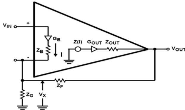
**Figure. 1: Generalized CFOA internal structure**
