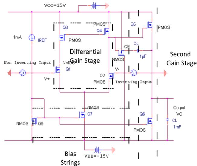
**Fig. 5 The schematic diagram of operational amplifier using CMOS**
