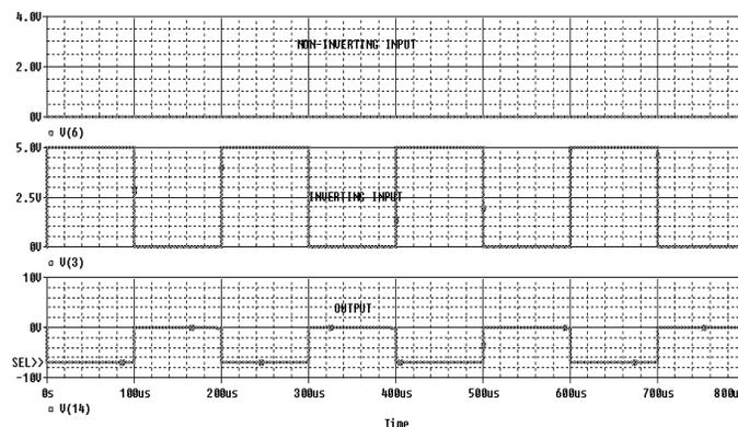
**Figure 9: Simulation results of Inverting Amplifier using CMOS**
