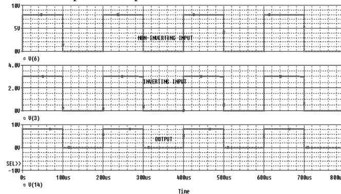
**Fig. 8: Simulation results of Differential Amplifier using BJT**
