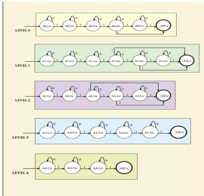
Fig 2. Finite State Machine for Addition
