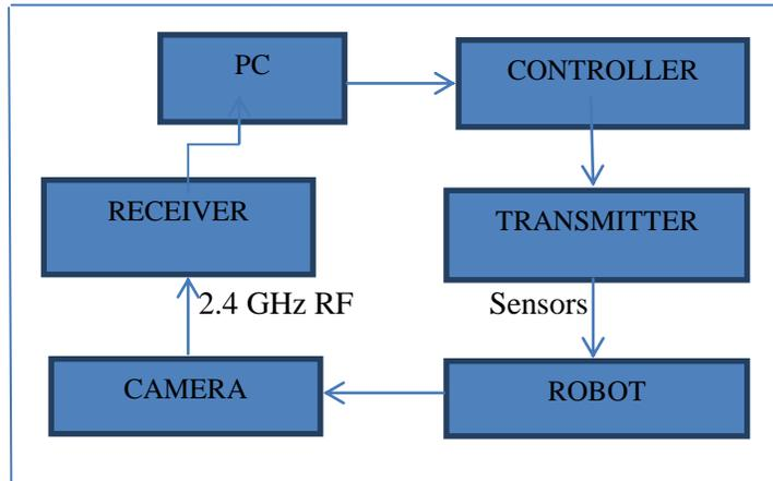
Figure 2: Block diagram of aerial robot
