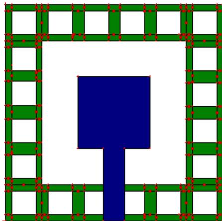
Fig. 3 Geometry of optimized antenna with scale factor,  $r=1/6$
