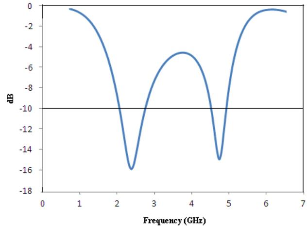
Fig. 4 Simulated s-parameters of optimized antenna
