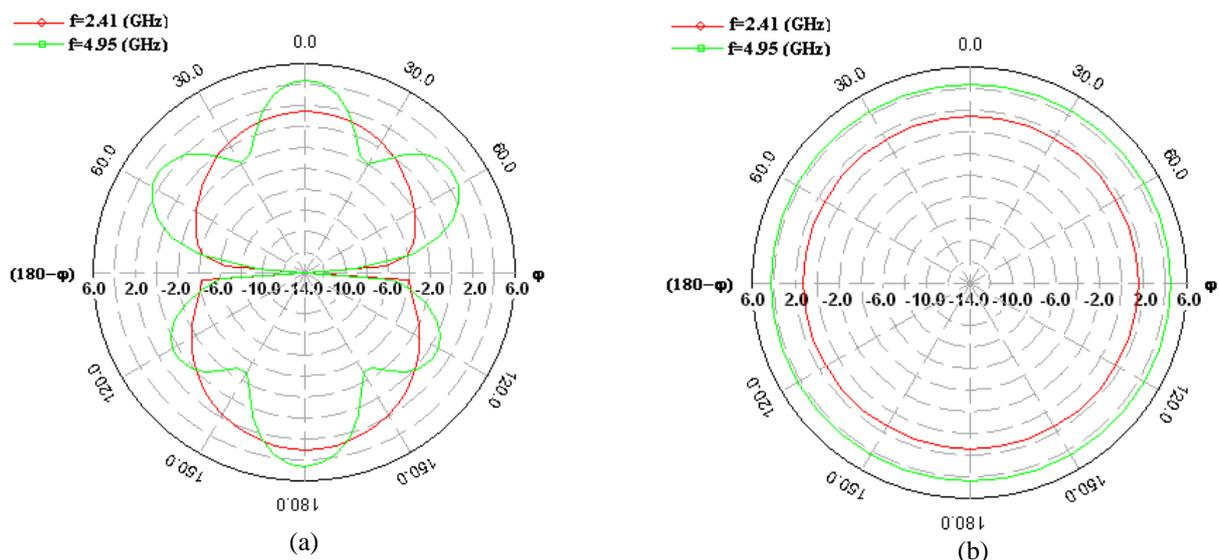
Fig. 5 Simulated radiation patterns of optimized antenna (a) E-plane (b) H-plane
