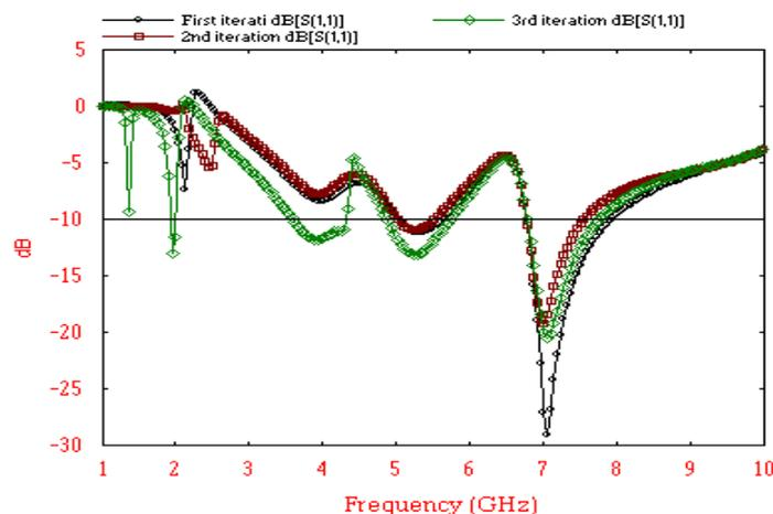
Fig. 2 Simulated s-parameters of all the three iterations
