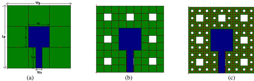
Fig. 1 Geometry of the proposed antenna (a) first iteration (b) second iteration (c) Third iteration
