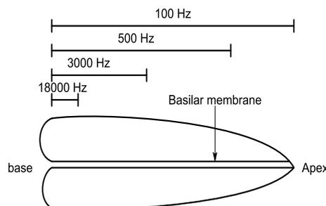
Fig. 2 Schematic of the basilar membrane, showing the change in characteristic frequency from base to apex.
