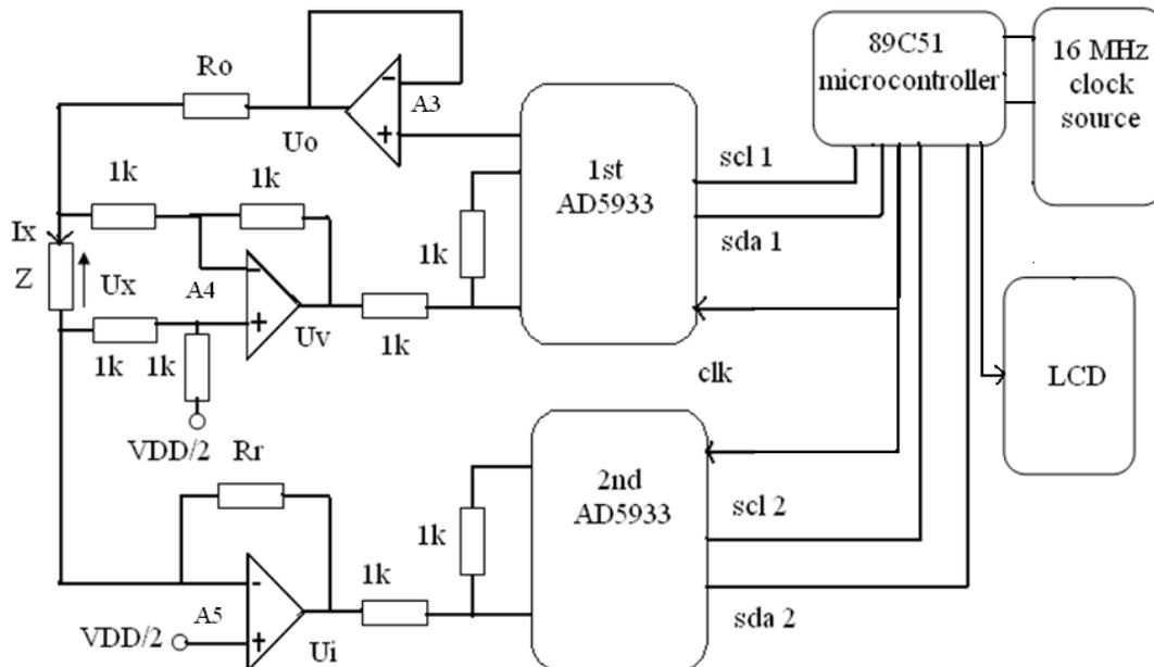
Fig.1 Schematic Diagram of the proposed system
