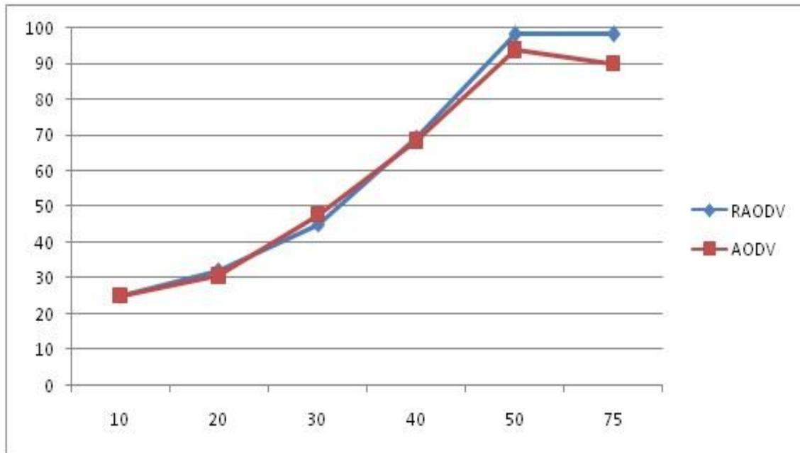
Figure 1: Packet Delivery ratio when number of node varies
