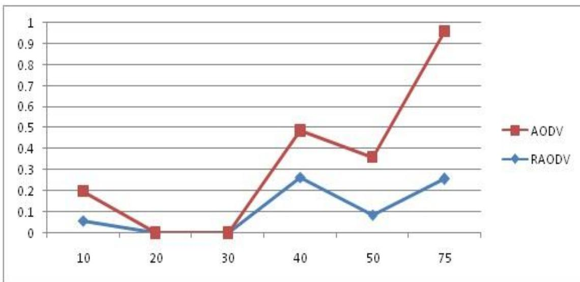
Figure 2: Average End to End delay when number of node varies
