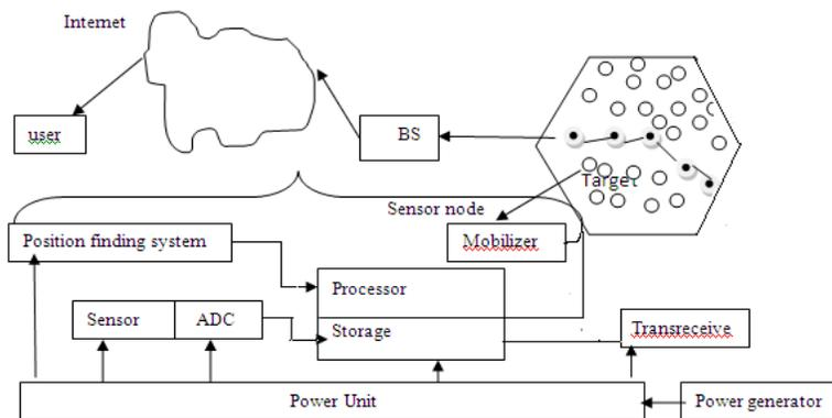
Figure 1. Sensor nodes scattered in a sensor field and components of a sensor node
