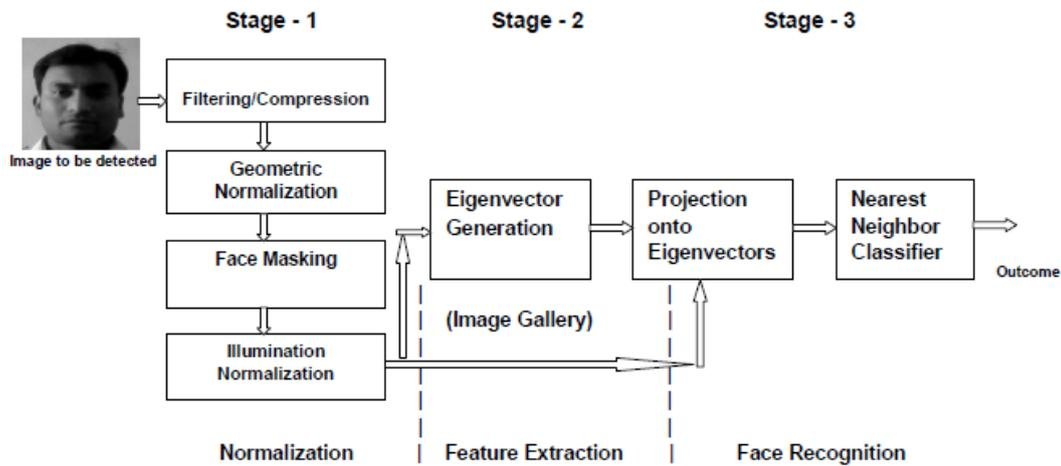
Figure 2 : Block diagram of PCA – based Face Recognition System.
