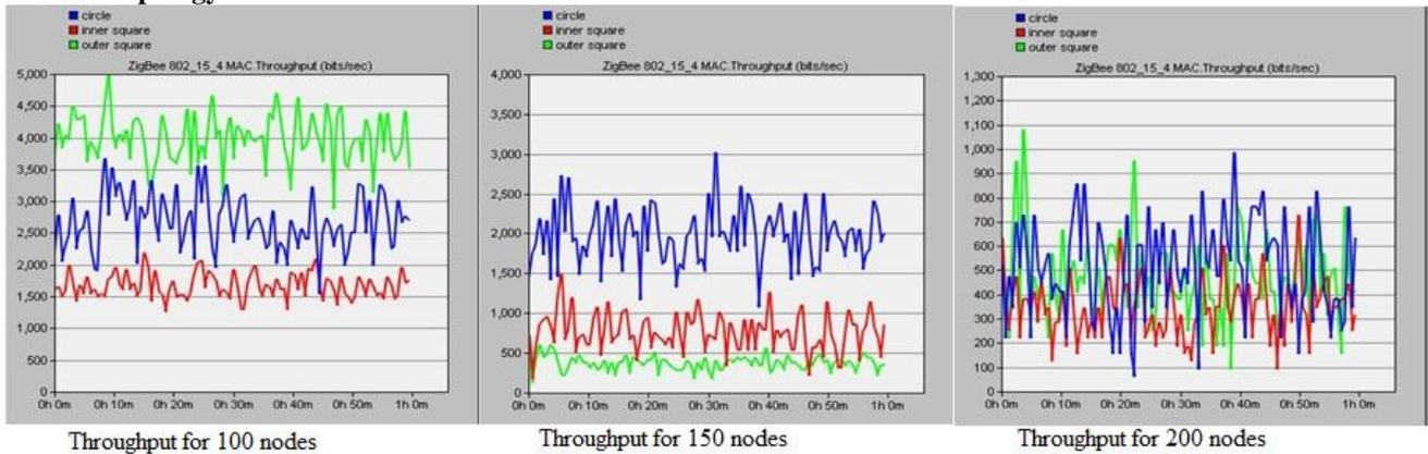
Figure 8: Throughput without ACK (tree)
