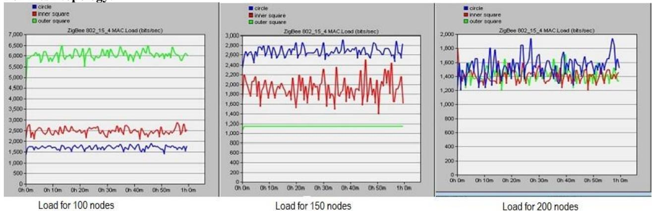
Figure 3: Load without ACK
