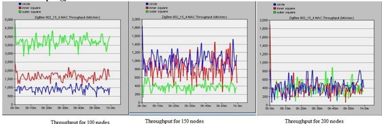
Figure 7: Throughput without ACK
