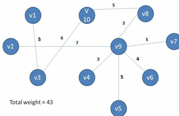
Fig. 4 Minimum Cost Spanning Tree-2 with 9 edges for the graph in Fig. 2
