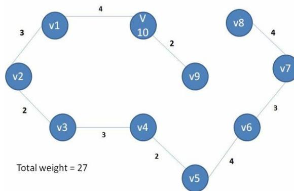
Fig. 3 Minimum Cost Spanning Tree -1 with 9 edges for the graph in Fig. 2
