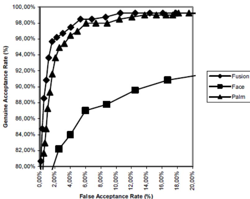
Figure 4: Comparison of unimodal and multimodal system verification results
