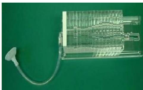
Fig. 3 Physical plate model of the human vocal tract
