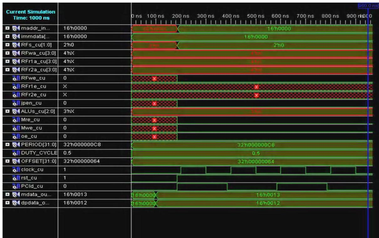
Fig.8 Simulation results for control unit
