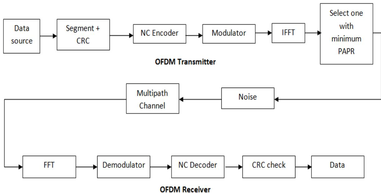
Figure1. Block Diagram of NC-SLM system
