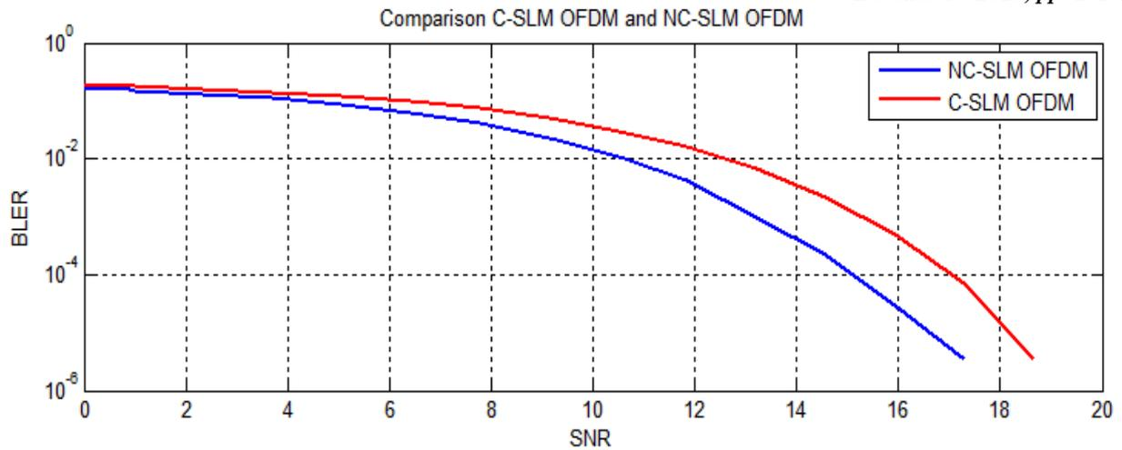
Figure 3. BLER performance of C-SLM and NC-SLM
