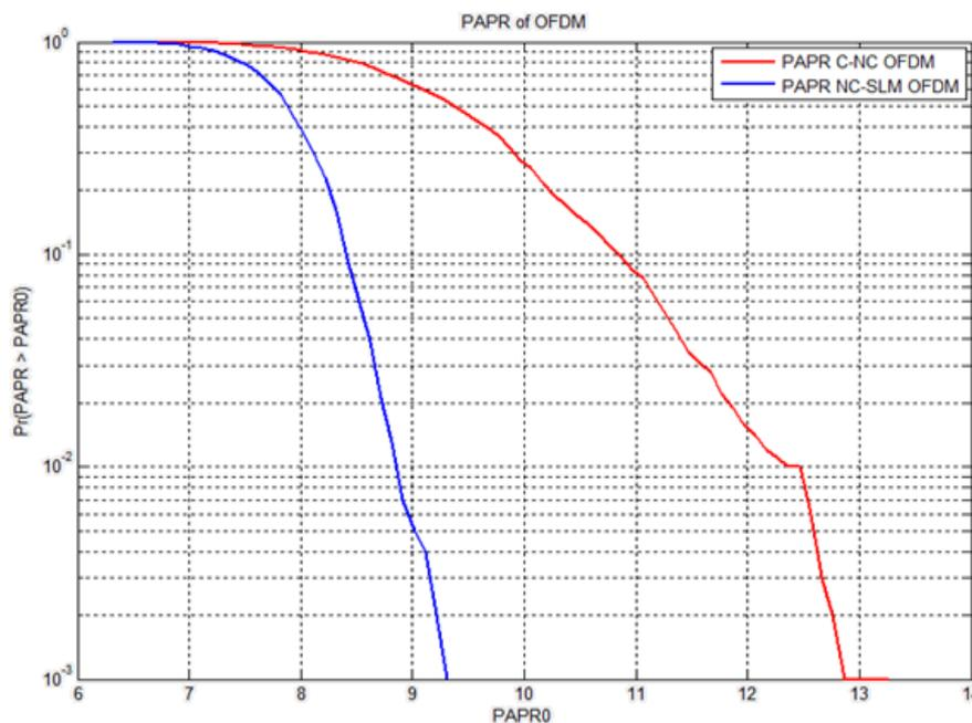
Figure 4. PAPR CCDF performance of C-SLM and NC-SLM schemes
