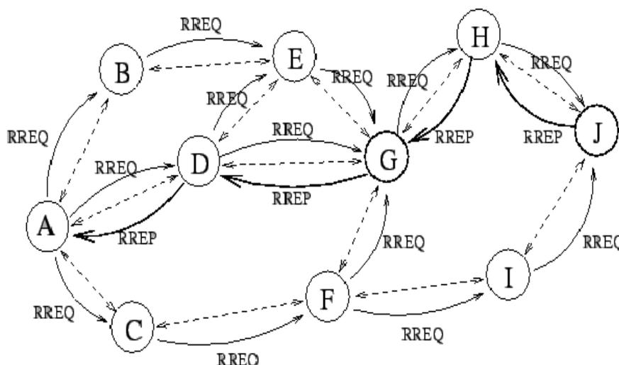
Figure 4 : Routing Process of AODV
