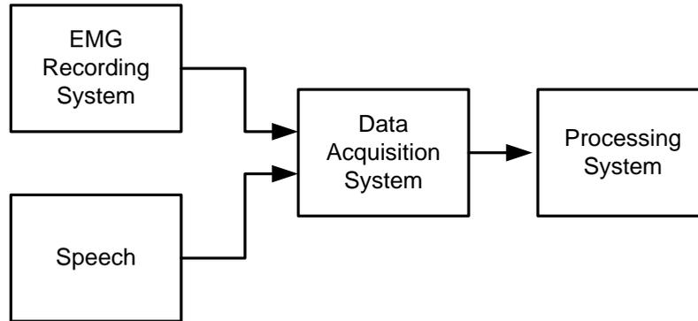
Fig. 3 Schematic block diagram for EMG signal acquisition
