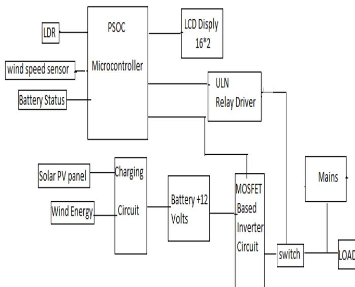
Fig. 4. Basic Block Diagram Of Self electricity Generation using Psoc
