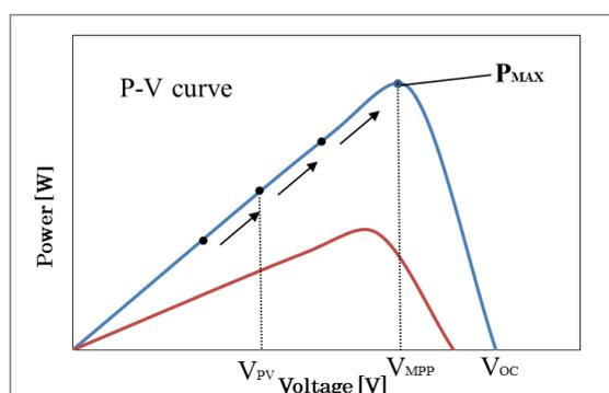
Fig.2 .Power-voltage characteristics of PV [1].
