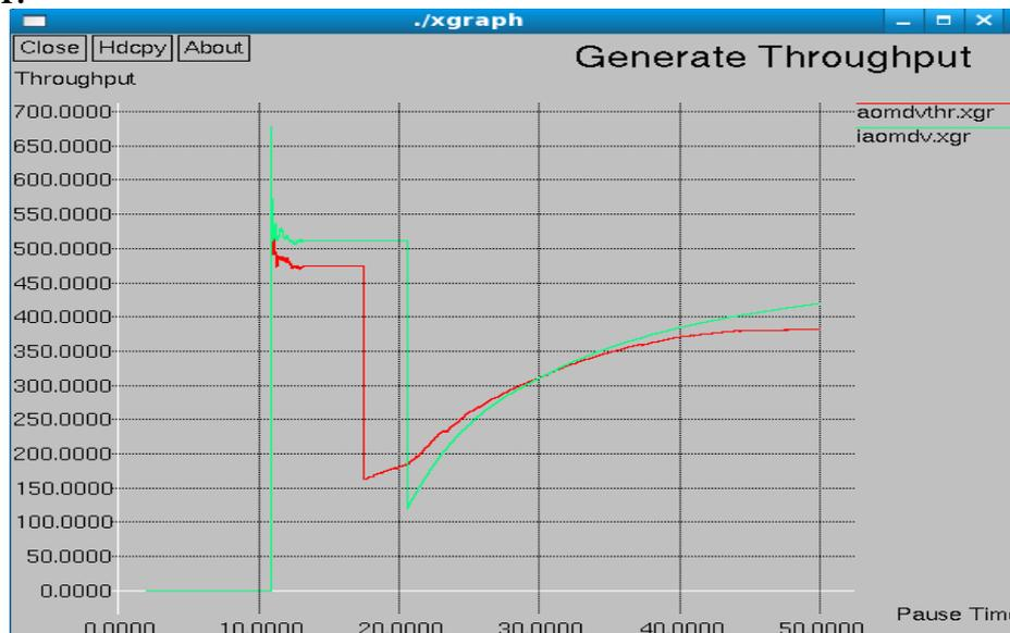
Fig.7 Xgraph shows Throughput comparison between AOMDV and I-AOMDV.
