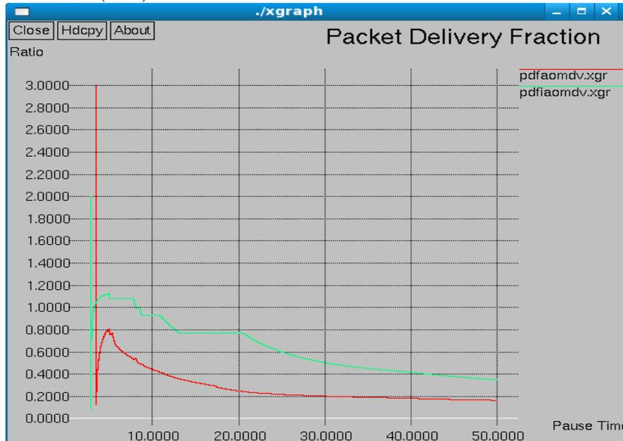
Fig.6 Xgraph shows Packet delivery Ratio comparison between AOMDV and I-AOMDV.
