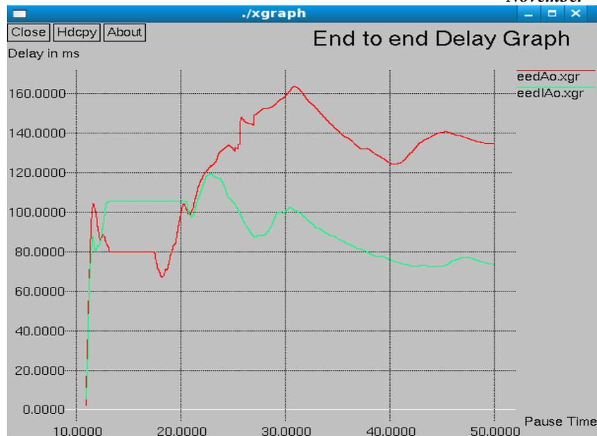
Fig.8 Xgraph shows End To End Delay comparison between AOMDV and I-AOMDV.
