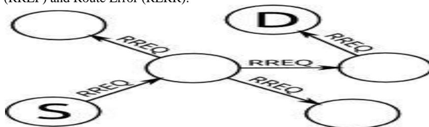
Fig 1: AODV packets routing pattern
