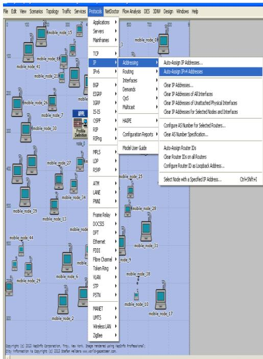
Fig 5: Auto assigning IPV4 addressing to all working nodes
