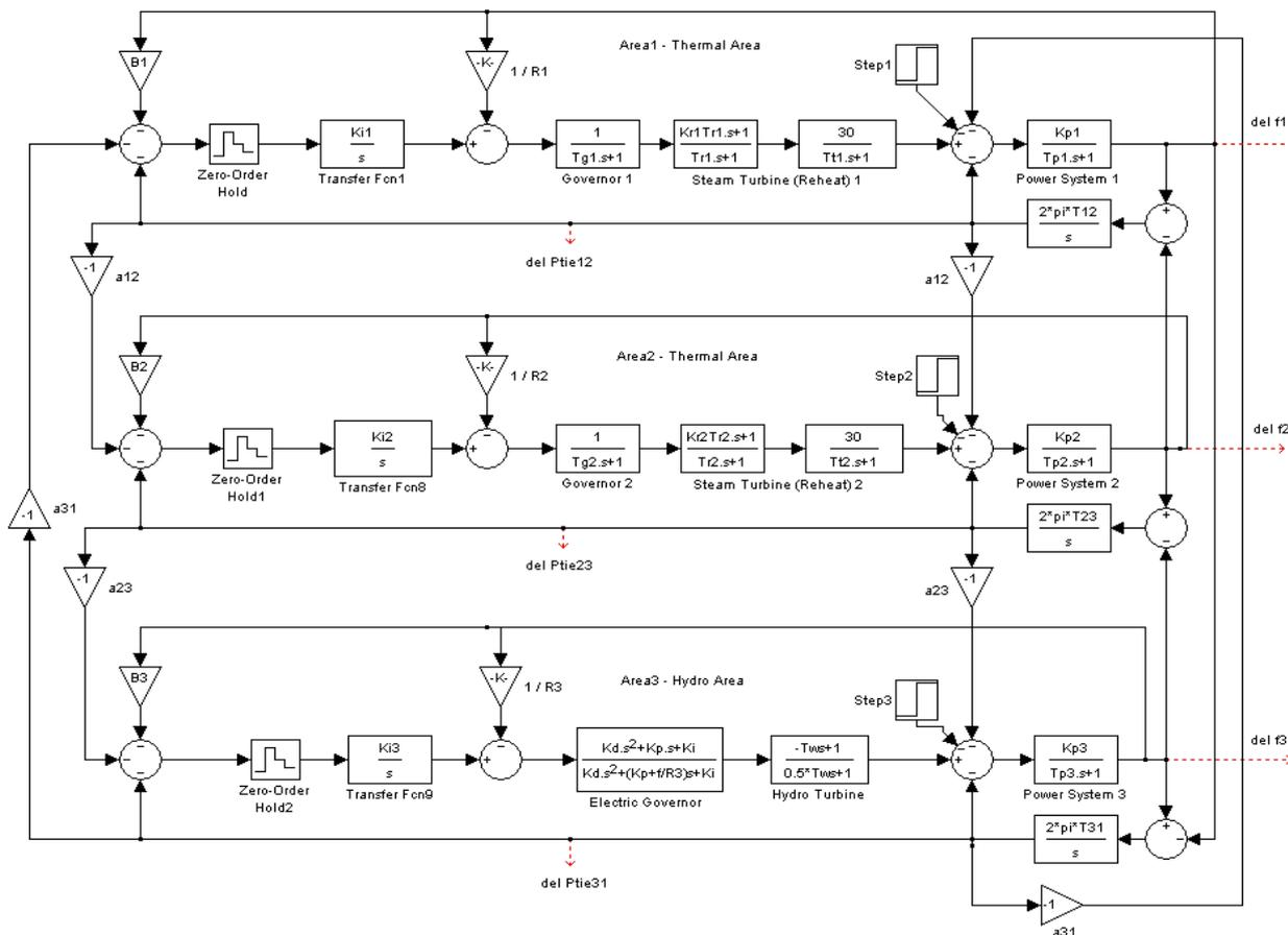
Fig 1. Transfer function model of three area thermal-thermal-hydro system
