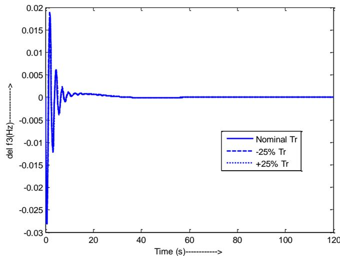
Fig 8. del f3 Vs time for different values of Tr.
