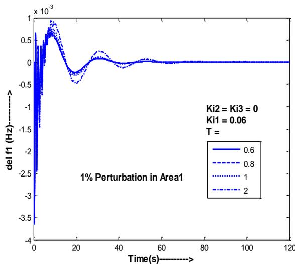
Fig 9. del f1 Vs time for different sampling times.
