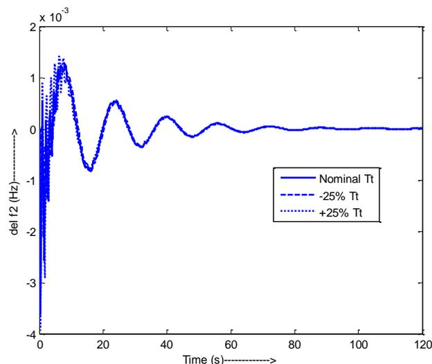
Fig 6.  $\delta f_2$  Vs time for different values of  $T_t$ .
