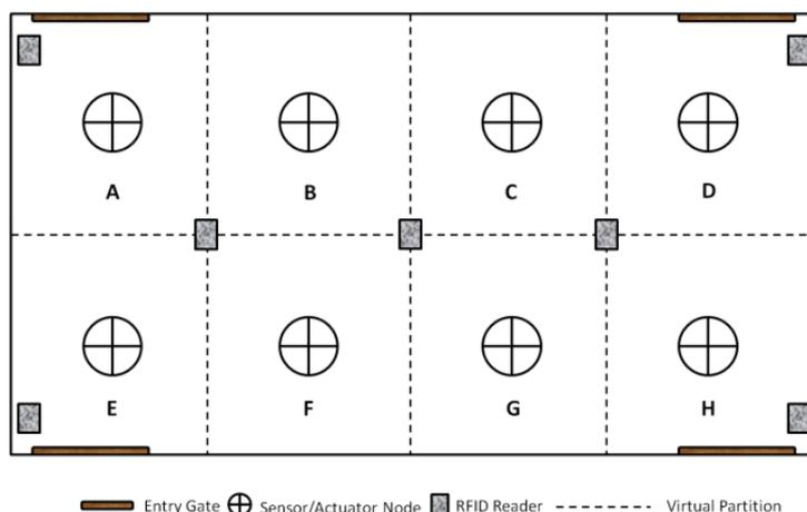
Fig 1: Layout of storage house with strategic placement of Sensors and RFID readers
