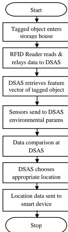
Fig 3: Flow chart of the process
