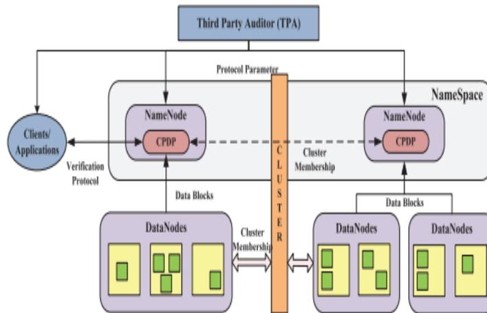
Fig .2: Applying CPDP scheme in Hadoop distributed file system
