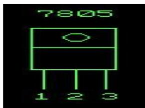
Fig 2: Pin diagram of I.C LM7805 [4]
