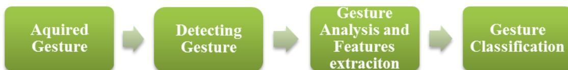
Fig 3 Recognition gesture system stages
