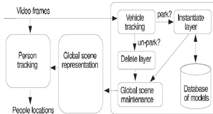
**Figure 4: Data representation enables tracking of pedestrians despite prolonged.**
