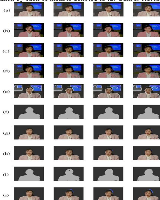
Figure 7: VOP generation for Akiyo video sequence using change information based scheme (for frames 75th, 95th, 115th, and 135th) (a) Original frames (b) Ground truth of original frames (c) Segmentation using proposed scheme (d) Segmentation using edgeless scheme (e) Segmentation using JSEG scheme (f) Temporal segmentation using label frame CDM (g) VOP generated by temporal segmentation result (f) (h) Centroid based tracking of VOPs as obtained in (g) (i) Temporal segmentation using original frame CDM (j) VOP generated by temporal segmentation result (i).
