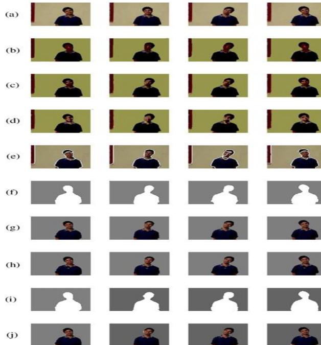
Figure 6: VOP generation for David video using change information based scheme (for frames 11th, 16th, 21st, and 26th) (a) Original frames (b) Ground truth of original frames (c) Segmentation using proposed scheme (d) Segmentation using edgeless scheme (e) Segmentation using JSEG scheme (f) Temporal segmentation using label frame CDM (g) VOP generated by temporal segmentation result (f); (h) Centroid based tracking of VOPs as obtained in (g); (i) Temporal segmentation using original frame CDM; (j) VOP generated by temporal segmentation result (i).
