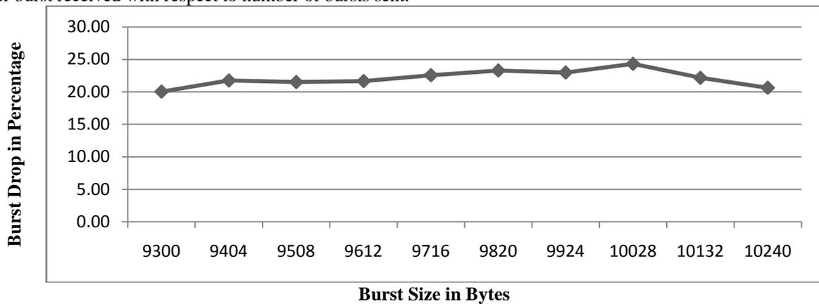
Fig 3: Burst Drop ratio for maximum burst length 20KB
