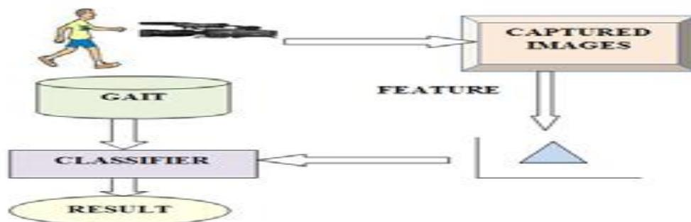
**Fig. 1: Block diagram of a gait recognition system.**
