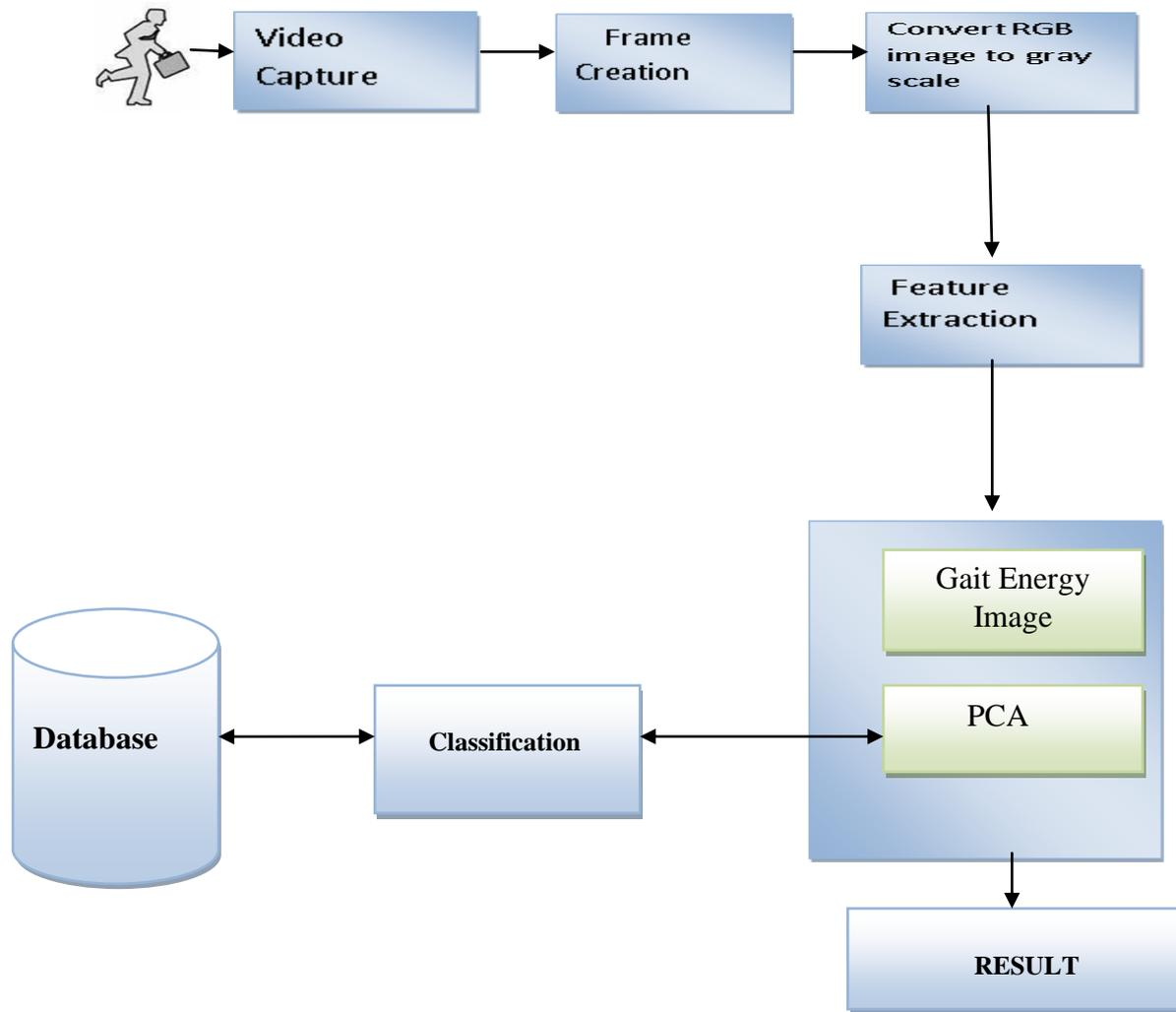
Figure 4: Block Diagram of the Proposed Gait System working
