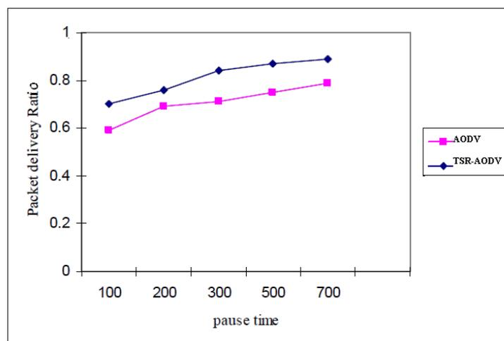
Fig.7 Packet Delivery Ratio at different pause time.
