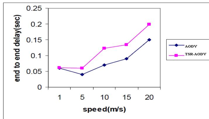
Fig.6 End to End delay at different speed.
