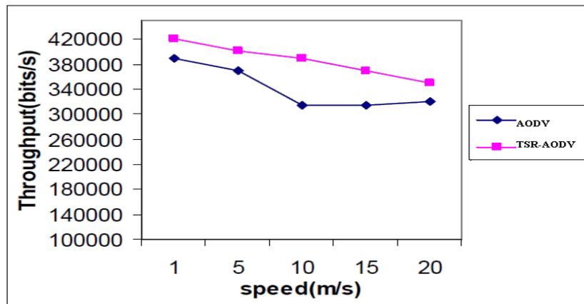
Fig.5 Throughput at different speed.
