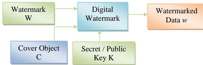
Fig 1 Digital Watermarking - Embedding Process
