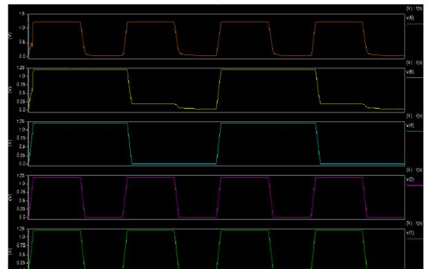
3. Simulation of 8 Transistor XOR Adder
