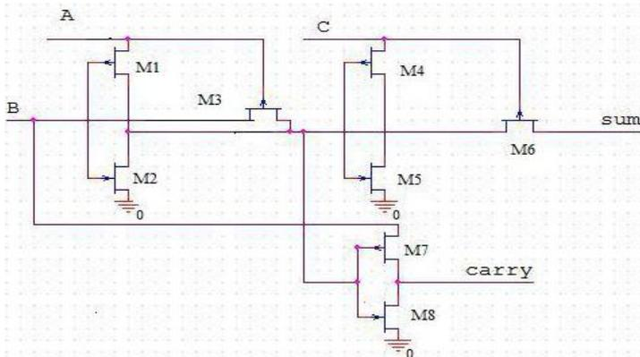
Fig. 1: Existing 8 Transistor XOR Full Adder
