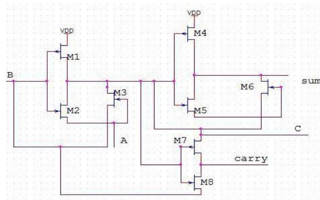
Fig. 2. – Proposed 8 Transistor XNOR Full Adder
