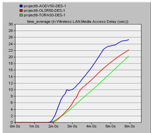
Fig 3.Media Access Delay (for 50 nodes)
