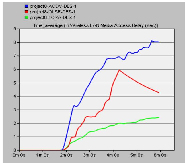
Fig 2.Media Access Delay (for 25 nodes)
