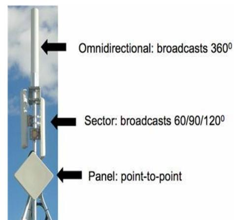
Figure 5: directional antenna
